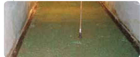
Post-test endurance results concluded that unvegetated GreenArmor 7020 exhibited a critical shear stress of 5.8 lb/ft 2 (276 N/m 2 ).
